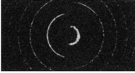
Fig. 2. Spectrograms of exciting (left) and scattered (right) radiation. The dispersion of the Fabry–Perot etalon is 3.33 \times 10^{-2} \text{ cm}^{-1}
